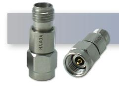
The HASCO Fixed Attenuator **HA40A-06** is rated to .5 Watts and operates from DC to 40 GHz. The versatile coaxial package uses 2.92 mm male to 2.92 mm female connectors.
