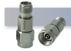
The HASCO Fixed Attenuator **HA40A-08** is rated to .5 Watts and operates from DC to 40 GHz. The versatile coaxial package uses 2.92 mm male to 2.92 mm female connectors.
