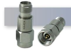
The HASCO Fixed Attenuator **HA40A-10** is rated to .5 Watts and operates from DC to 40 GHz. The versatile coaxial package uses 2.92 mm male to 2.92 mm female connectors.
