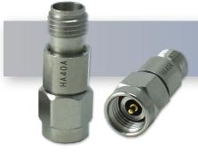
30 dB - Fixed Attenuator 2.92 mm Male To 2.92mm Female Up To 40 GHz Rated To .5 Watts with Passivated Stainless Steel Body
