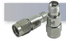
The HASCO Fixed Attenuator **HA40A2-01** is rated to 2 Watts and operates from DC to 40 GHz. The versatile coaxial package uses 2.92 mm male to 2.92 mm female connectors.
