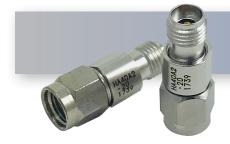
The HASCO Fixed Attenuator **HA40A2-03** is rated to 2 Watts and operates from DC to 40 GHz. The versatile coaxial package uses 2.92 mm male to 2.92 mm female connectors.
