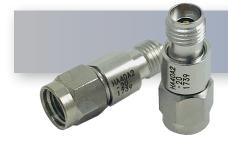
The HASCO Fixed Attenuator **HA40A2-05** is rated to 2 Watts and operates from DC to 40 GHz. The versatile coaxial package uses 2.92 mm male to 2.92 mm female connectors.
