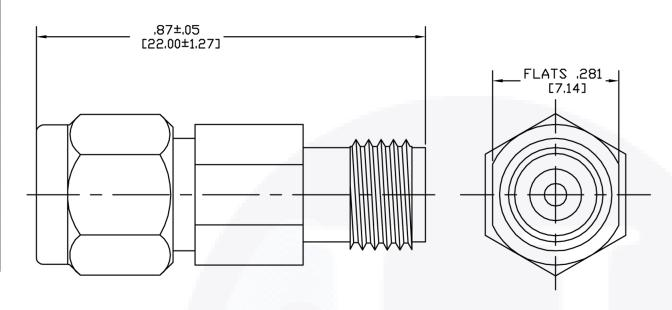
To view online, go to: <a href="https://www.hasco-inc.com/attenuators/8-db-fixed-attenuator-2-92mm-male-to-2-92mm-female-up-to-40-ghz-rated-to-2-watts-with-passivated-stainless-steel-body/">https://www.hasco-inc.com/attenuators/8-db-fixed-attenuator-2-92mm-male-to-2-92mm-female-up-to-40-ghz-rated-to-2-watts-with-passivated-stainless-steel-body/</a>
