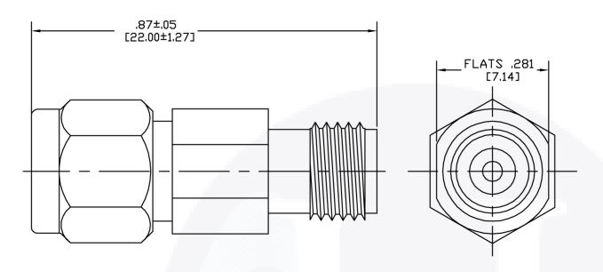
To view online, go to: <a href="https://www.hasco-inc.com/attenuators/9-db-fixed-attenuator-2-92mm-male-to-2-92mm-female-up-to-40-ghz-rated-to-2-watts-with-passivated-stainless-steel-body/">https://www.hasco-inc.com/attenuators/9-db-fixed-attenuator-2-92mm-male-to-2-92mm-female-up-to-40-ghz-rated-to-2-watts-with-passivated-stainless-steel-body/</a>
