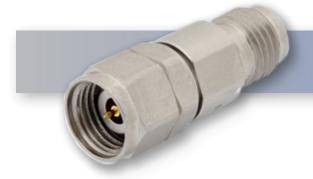
The HASCO **HA50A-XX** is a 2.4mm Male to Female Attenuator manufactured by HASCO. This type of Attenuator is bidirectional. Attenuators like this HA50A-XX are used to reduce or step down the power level of a signal while maintaining the waveforms integrity. The operating frequency for this model is DC to 50 GHz.
