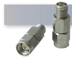
The HASCO **HA6A-02** is an RF attenuator that operates from DC to 6 GHz and handles up to 2 Watts (CW). This attenuator is constructed with SMA Male to SMA Female connectors. The HA6A-02 Attenuator offers 1.20:1 max VSWR.
