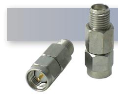
The HASCO **HA6A-07** is an RF attenuator that operates from DC to 6 GHz and handles up to 2 Watts (CW). This attenuator is constructed with SMA Male to SMA Female connectors. The HA6A-07 Attenuator offers 1.25:1 max VSWR.
