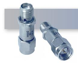
The HASCO **HA6A2-20** is an RF attenuator that operates from DC to 6 GHz and handles up to 2 Watts (CW). This attenuator is constructed with SMA Male to SMA Female connectors. The HA6A2-20 Attenuator offers 1.20:1 max VSWR.
