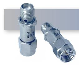
The HASCO **HA6A2-30** is an RF attenuator that operates from DC to 6 GHz and handles up to 2 Watts (CW). This attenuator is constructed with SMA Male to SMA Female connectors. The HA6A2-30 Attenuator offers 1.20:1 max VSWR.
