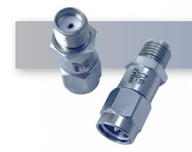
The HASCO HA6A2-05 is an RF attenuator that operates from DC to 6 GHz and handles up to 2 Watts (CW). This attenuator is constructed with SMA Male to SMA Female connectors. The HA6A2-05 Attenuator offers 1.20:1 max VSWR.
