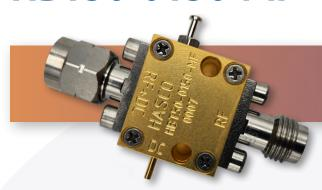
The HASCO **HBT50-0150-MF** is a 50 GHz Bias Tee with 2.4mm Female to 2.4mm Male connectors.
