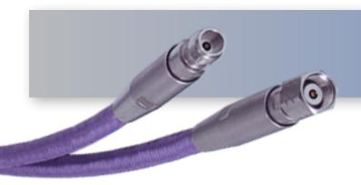
1.85mm Male to 1.85mm FemaleTest Cable using LL185 Low Loss Ruggedized Flexible Cable, Excellent Phase and Amplitude Stability vs. Flexure, DC-67 GHz, 24 Inches
