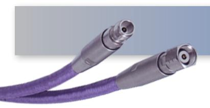
1.85mm Male to 1.85mm FemaleTest Cable using LL185 Low Loss Ruggedized Flexible Cable, Excellent Phase and Amplitude Stability vs. Flexure, DC-67 GHz, 30 Inches
