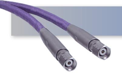
The HASCO **HLL185R Series Cable** is a low loss LL185 cable that operates from DC to 67 GHz. This cable series is constructed with 1.85mm Male to 1.85mm Male connectors. These cables are internally ruggedized with multi-layer copper spiral and braided armor. They offer excellent phase and amplitude stability vs. flexure. The HLL185R Series cables offer 1.50:1 max VSWR.
