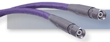
The HASCO HLL185R Series Cable is a low loss LL185 cable that operates from DC to 67 GHz. This cable series is constructed with 1.85mm Male to 1.85mm Male connectors. These cables are internally ruggedized with multi-layer copper spiral and braided armor. They offer excellent phase and amplitude stability vs. flexure. The HLL185R Series cables offer 1.50:1 max VSWR.
