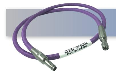
2.4mm Male to 2.4mm FemaleTest Cable using LL228 Low Loss Ruggedized Flexible Cable, Excellent Phase and Amplitude Stability vs. Flexure, DC-50 GHz, 24 Inches
