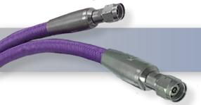
The HASCO HLL228R Series Cable is a low loss LL228 cable that operates from DC to 50 GHz. This cable series is constructed with 2.4mm Male to 2.4mm Female connectors. These cables are internally ruggedized with multi-layer copper spiral and braided armor. They offer excellent phase and amplitude stability vs. flexure. The HLL228R Series cables offer 1.35:1 max VSWR.
