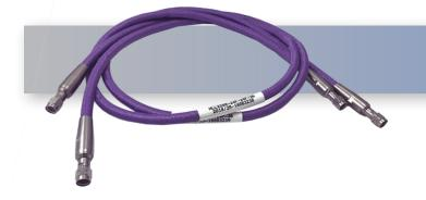
The HASCO **HLL228R** Series Cable is a low loss LL228 cable that operates from DC to 50 GHz. This cable series is constructed with 2.4mm Male to 2.4mm Male connectors. These cables are internally ruggedized with multi-layer copper spiral and braided armor. They offer excellent phase and amplitude stability vs. flexure.
