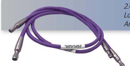
The HASCO **HLL228R Series Cable** is a low loss LL228 cable that operates from DC to 50 GHz. This cable series is constructed with 2.4mm Male to 2.4mm Male connectors. These cables are internally ruggedized with multi-layer copper spiral and braided armor. They offer excellent phase and amplitude stability vs. flexure. The
