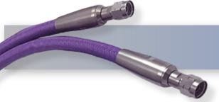
The HASCO HLL228R Series Cable is a low loss LL228 cable that operates from DC to 50 GHz. This cable series is constructed with 2.4mm Male to 2.4mm Male connectors. These cables are internally ruggedized with multi-layer copper spiral and braided armor. They offer excellent phase and amplitude
