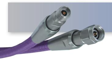
The HASCO **HLL228R Series Cable** is a low loss LL228 cable that operates from DC to 40 GHz. This cable series is constructed with 2.92mm Male to 2.92mm Female connectors. These cables are internally ruggedized with multi-layer copper spiral and braided armor. They offer excellent phase and amplitude stability vs. flexure. This HLL228R Series cables offers 1.30:1 max VSWR.
