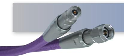
The HASCO **HLL228R Series Cable** is a low loss LL228 cable that operates from DC to 40 GHz. This cable series is constructed with 2.92mm Male to 2.92mm Female connectors. These cables are internally ruggedized with multi-layer copper spiral and braided armor. They offer excellent phase and amplitude stability vs. flexure. This HLL228R Series cables offers 1.30:1 max VSWR.
