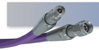
The HASCO **HLL228R Series Cable** is a low loss LL228 cable that operates from DC to 40 GHz. This cable series is constructed with 2.92mm Male to 2.92mm Female connectors. These cables are internally ruggedized with multi-layer copper spiral and braided armor. They offer excellent phase and amplitude stability vs.
