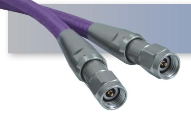
The HASCO **HLL228R Series Cable** is a low loss LL228 cable that operates from DC to 40 GHz. This cable series is constructed with 2.92mm Male to 2.92mm Male connectors. These cables are internally ruggedized with multi-layer copper spiral and braided armor. They offer excellent phase and amplitude stability vs. flexure. This HLL228R Series cables offers 1.30:1 max VSWR.
