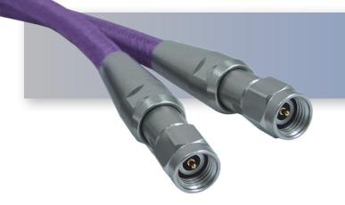
The HASCO **HLL228R Series Cable** is a low loss LL228 cable that operates from DC to 40 GHz. This cable series is constructed with 2.92mm Male to 2.92mm Male connectors. These cables are internally ruggedized with multi-layer copper spiral and braided armor. They offer excellent phase and amplitude stability vs. flexure. This HLL228R Series cables offers 1.30:1 max VSWR.
