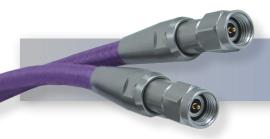
The HASCO HLL228R Series Cable is a low loss LL228 cable that operates from DC to 40 GHz. This cable series is constructed with 2.92mm Male to 2.92mm Male connectors. These cables are internally ruggedized with multi-layer copper spiral and braided armor. They offer excellent phase and amplitude stability vs. flexure. The HLL228R Series cables offer 1.30:1 max VSWR.
