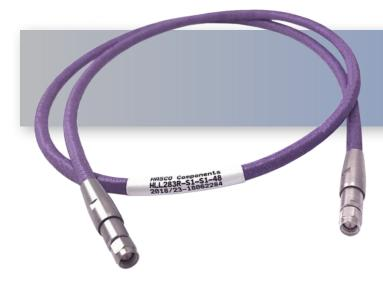
The HASCO **HLL283R Series Cable** is a low loss LL283 cable that operates from DC to 26.5 GHz. This cable series is constructed with SMA Male to SMA Male connectors. These cables are internally ruggedized with multi-layer copper spiral and braided armor. They offer excellent phase and amplitude stability vs. flexure. The HLL283R Series cables offer 1.30:1 max VSWR.
