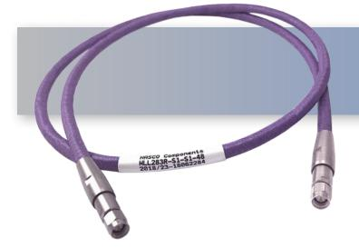
The HASCO **HLL283R Series Cable** is a low loss LL283 cable that operates from DC to 26.5 GHz. This cable series is constructed with SMA Male to SMA Male connectors. These cables are internally ruggedized with multi-layer copper spiral and braided armor. They offer excellent phase and amplitude stability vs. flexure. The HLL283R Series cables offer 1.30:1 max VSWR.
