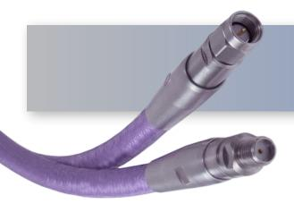
The HASCO **HLL283R Series Cable** is a low loss LL283 cable that operates from DC to 26.5 GHz. This cable series is constructed with SMA Male to SMA Female connectors. These cables are internally ruggedized with multi-layer copper spiral and braided armor. They offer excellent phase and amplitude stability vs. flexure. The HLL283R Series cables offer 1.30:1 max VSWR.
