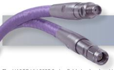
The HASCO HLL283R Series Cable is a low loss LL283 cable that operates from DC to 26.5 GHz. This cable series is constructed with SMA Male to SMA Female connectors. These cables are internally ruggedized with multi-layer copper spiral and braided armor. They offer excellent phase and amplitude stability vs. flexure. The HLL283R Series cables offer 1.30:1 max VSWR.
