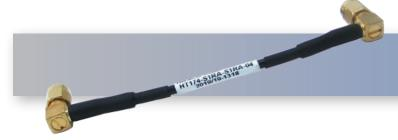
The HASCO **HT174** flexible cables are terminated with high quality SMA straight or SMA right angle connectors. Standard connectors are SMA Male Straight (S1) and SMA Right Angle (S1RA). Additional configurations available by special order.
