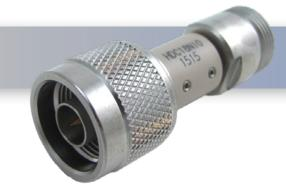
The **HDC18NIO** is a Type N DC Block, inner and Outer design from HASCO. The Type N Male to Type N Female DC Block will operate from 10 MHz to 65 GHz with a maximum voltage of 200V (Inner and Outer).
