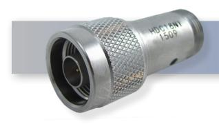
The HASCO **HDC18NI** is a DC Block with Type N Male to Type N Female connectors (inner only) from HASCO. This DC Block will operate from 10 MHz 18 GHz.
