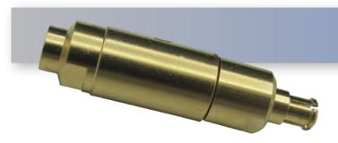
The **HDC26SMPPI-FD** is a SMP DC Block, inner only design from HASCO. The SMP Male to SMP Female Full Detent DC Block will operate from 1.35 MHz to 26.5 GHz with a maximum voltage of 50V.
