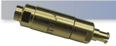
The **HDC26SMPPI-LD** is a SMP DC Block, inner only design from HASCO. The SMP Male to SMP Female Limited Detent DC Block will operate from 1.35 MHz to 26.5 GHz with a maximum voltage of 50V.
