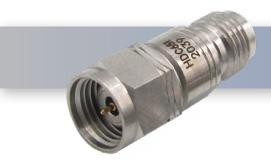
The **HDC65I** is a 1.85mm DC Block, inner only design from HASCO. The 1.85mm Male to 1.85mm Female DC Block will operate from 10 MHz to 65 GHz with a maximum input power of 1 Watt and maximum voltage of 16V.
