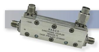
The HASCO **HC0220-10** is an SMA Female Directional Coupler that operates from 2 to 20 GHz from HASCO. This Coupler has low insertion loss at 1.5 dB Max and flatness rating of 0.85 dB Max.
