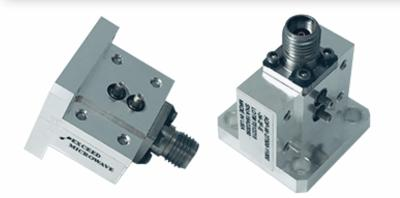
The ADP-W-27500-11000-34-2F-E is a WR-34 to 2.92mm female waveguide to coax adapter which operates across the entire WR-34 frequency band of 22 GHz to 33 GHz with return loss of 20dB minimum. WR-34/UG1530/U Flange.
