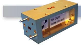
The BPF-WH1-60000-500-4-15 is a WR-15 V-Band Band-pass Filter with narrow pass-band. It is a 4 section filter with 1.7dB insertion loss. It is 1.7 inches in length. Input and outpur are WR-15 UG385/U.
