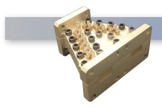
The DPX-WC-22-28-34 is a WR-34 Ka-Band diplexer at 20.33-24.33 GHz & 25.9-31.3 GHz with very wide bandwidth for both channels. Both channels provide 20% bandwidth with low insertion loss and low VSWR. Together, both channels cover nearly the entire WR34 waveguide band. It is very compact, nearly half the size of typical waveguide diplexers. Input and output are WR-34 UG1530.
