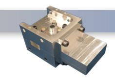
The ISO-W-19000-4000-51 is a WR-51 K-Band Isolator with passband from 18-21 GHz. It provides very low insertion loss <0.15dB and >22dB return loss.
