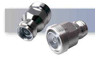
4.3-10 Female to 7/16 Female Between-Series Low PIM RF adapter, -168 dBc PIM Level from DC - 6 GHz
