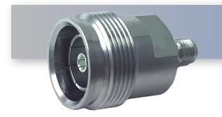
The 4310J-SMAJ-SLP is a 4.3-10 Female to SMA Female Between-Series Low PIM RF adapter, -165 dBc PIM Level from DC - 6 GHz manufactured by HASCO Components.
