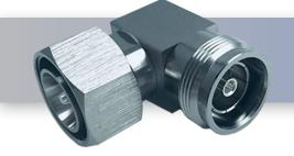
4.3-10 Male to 4.3-10 Female Right Angle In-Series Low PIM RF adapter, -165 dBc PIM Level from DC - 6 GHz
