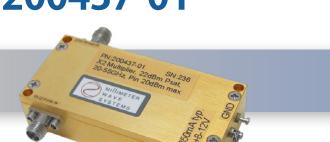
Active Frequency Multipliers use state-of-the-art active multiplier devices for frequency multiplication and amplification. The standard housing enables I/O ports of 2.4mm and 2.92mm (SMA Compatible) coaxial connectors. Featuring convenient single +8V supply operation, internally bias sequenced and regulated. This active multiplier from Millimeter Wave Systems offers high-output at +22 dBm with excellent fundamental rejection.
